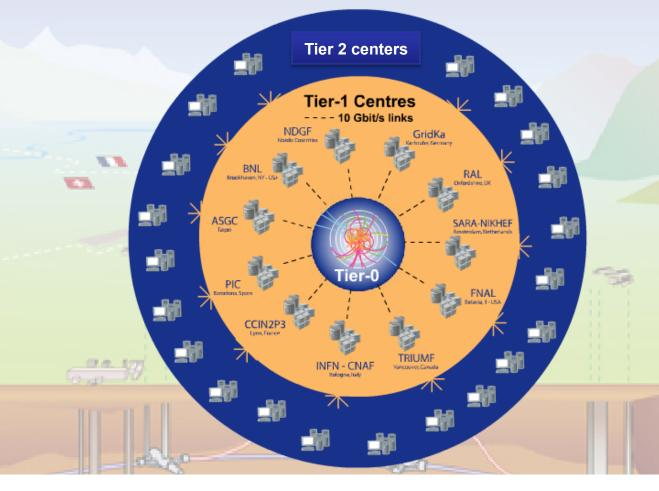
Tier-0 (CERN): • Data recording • Initial data reconstruction • Data distribution Tier-1 (11 centers): • Permanent storage • Re-processing • Analysis Tier-2 (>200 centers)
