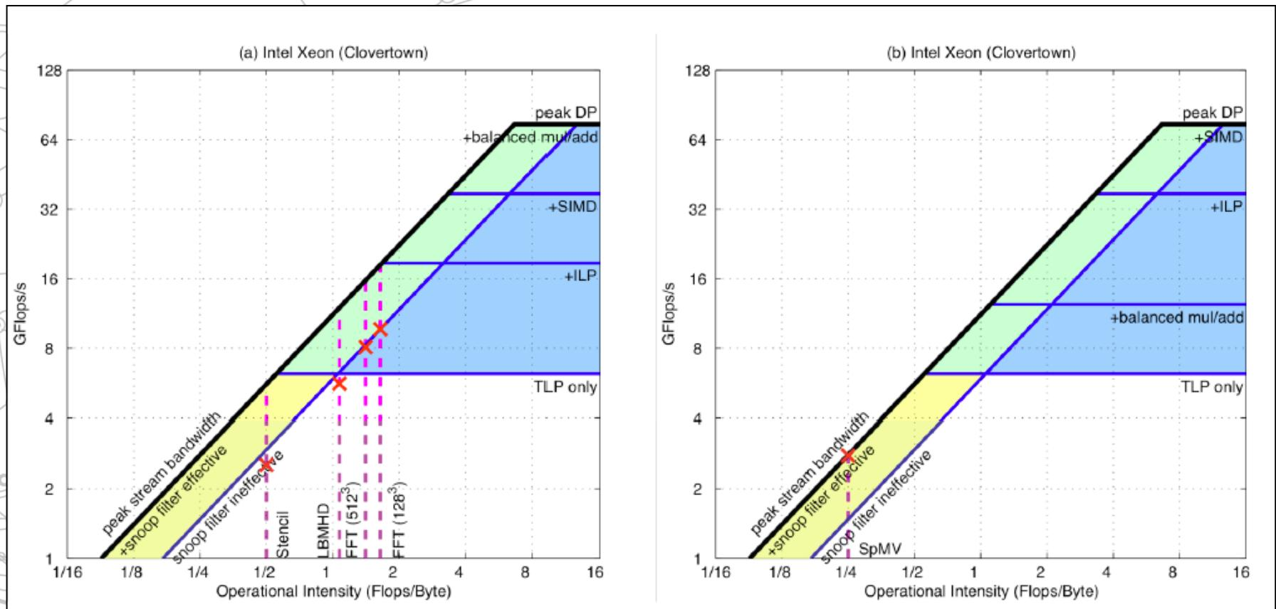
Roofline Model for Intel Xeon Processor
