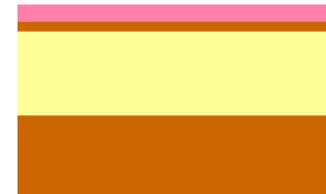
step5: pattern PhotoResist
