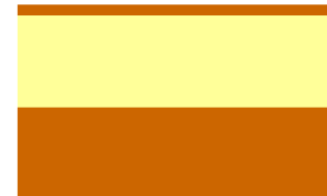
step4: PhotoResist deposit
