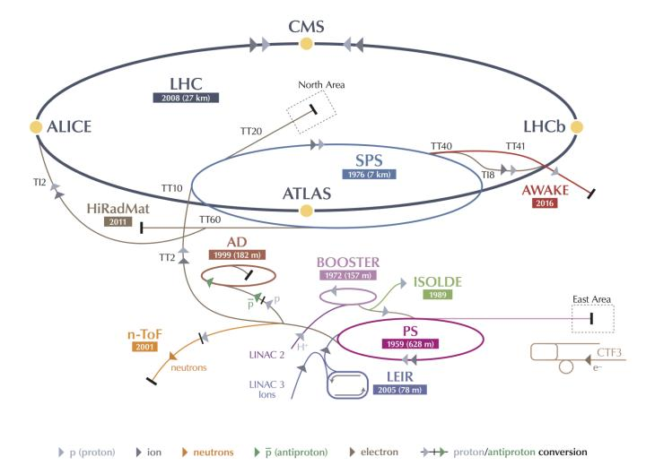
LHC Large Hadron Collider SPS Super Proton Synchrotron PS Proton Synchrotron
