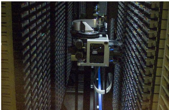
A robot manages some of CERN's 50PB of tape storage.
