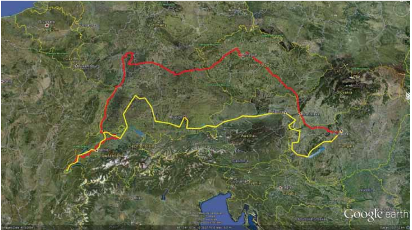
Two redundant high-speed links (100 gigabits per second) connect CERN data centre to its extension hosted in Hungary at the Wigner Research Centre for Physics.
